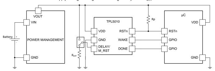
Figure 12. Manual Reset with SPDT Switch
