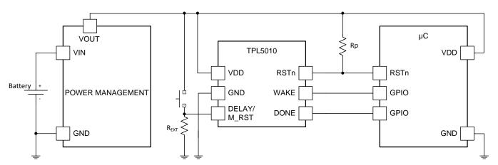
Figure 11. Manual Reset with SPST Switch
